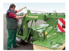
**Cutting height control** Cranks set the cutting height steplessly and separately on each unit.
