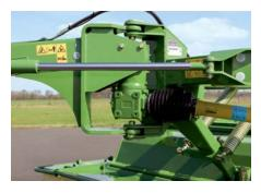
**Frictional connections without belts** The drive power flows via overload protected gearboxes and drive shafts to power the cutterbar and conditioner. Two swivel gearboxes optimize the flow down the drive shafts.
