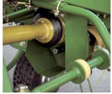
Narrow windrowing gearbox This optional gearbox is simply pushed on the shaft and reduces the rotor speed to produce narrow night windrows.
