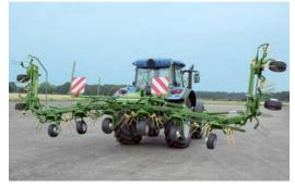
**Wide becomes narrow** The rotors are folded hydraulically. The outer rotors swing in to reduce the machine's transport height.
