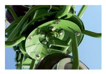
**Tedding at a steep angle, turning at a shallow angle** Setting the angle from 13 to 19 degrees is an easy job, which is carried out quickly on a pin-and-hole system on the brackets that hold the wheel arms. The steep position is preferred during tedding; the shallow position is best for turning.
