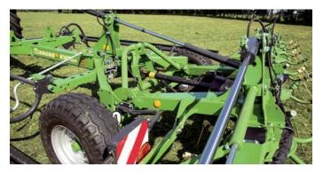
Accurate guidance The bottom arms on the chassis give very accurate guidance of the rotors.
