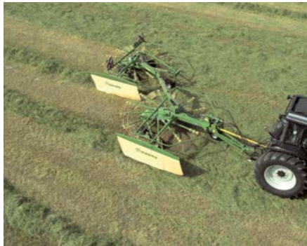
Forming two windrows Raking 6.80 m (22'4") into two windrows
